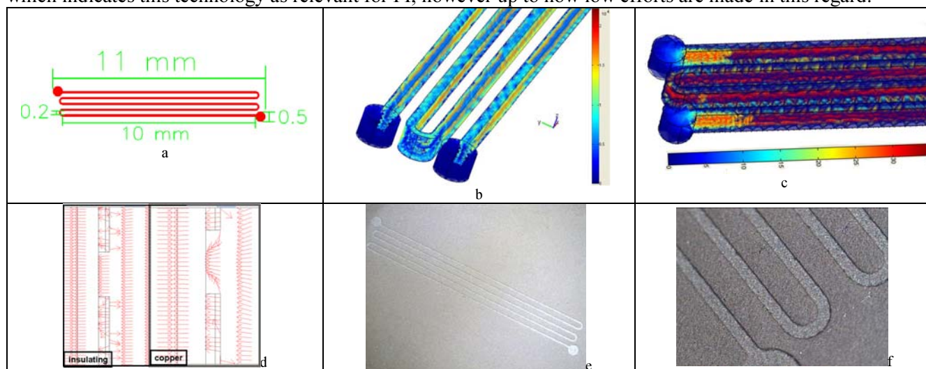
Fig. 1. Microchannels: (a) CAD; (b) vorticity ( s^{-1} ) on channels 10 mm length distant 200 \mu\text{m} ; (c) velocity (cm/s) on channels 20 mm length distant 200 \mu\text{m} ; (d) electric field on insulating and copper channels; (e), (f) photos of the channel
