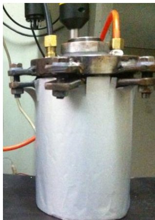
Fig. 1. Image system, showing gas inlet (black hose) and outlet (red orange hose) in addition to part of the Pirani gauge at the cathode.
