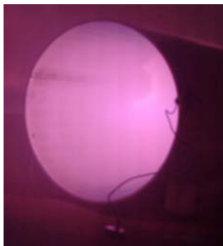
Fig. 1 Hollow cathode plasma in 16cm \emptyset tube
